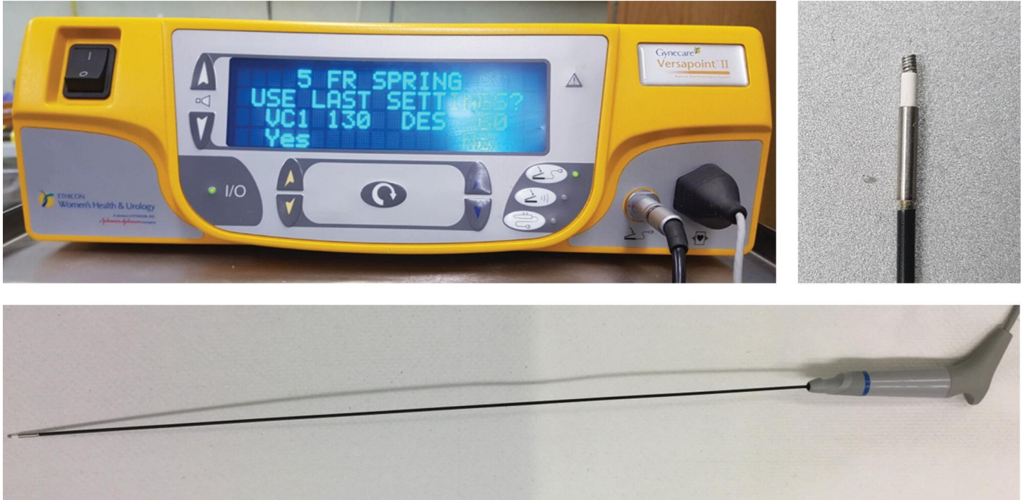
Fig. 37.3 Versapoint Bipolar Electrosurgery System™ (Ethicon, USA). Spring-tip electrode suitable for removing polyps, and grade 0 fibroids) is shown with the electrosurgical generator. A needle-like twizzle-tip electrode is also available (not shown) for removing polyps, septa, and adhesions.
